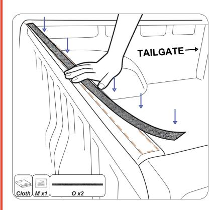
Clean any dust or dirt from top front edges of Ute tub with clean cloth and then wipe down with surface cleaning wipe. Let the surface dry. Then apply Velcro strips with even firm pressure.
