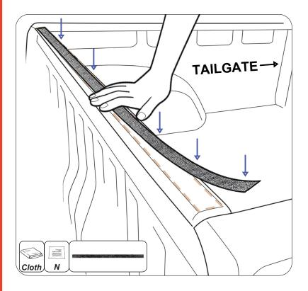
Clean any dust or dirt from top front edge of UTE tub with clean cloth and then wipe down with surface cleaning wipe. Let the surface dry. Then apply Velcro strip with **even firm pressure**. **Allow to cure for 24 hours for full bond strength.**
