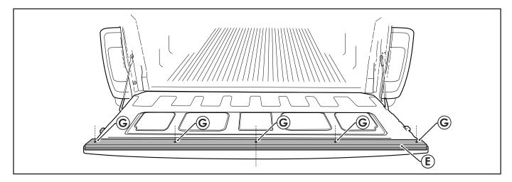
• Remove the red tape from back of the Tailgate Rail  $\bigcirc$ . Then stick the Tailgate Rail centrally onto the tailgate. Drill with a 4mm drill bit through the 5 holes. Apply rust inhibitor  $\bigcirc$  and then rivet  $\bigcirc$  the Tailgate Rail to the tailgate using a rivet gun.
