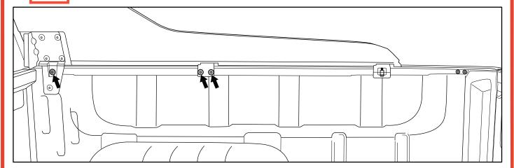
• Remove the three factory screws pointed above with T45 torx bit.
