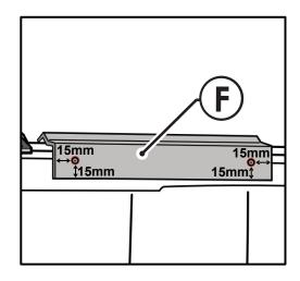
• Use above dimension guidance to drill holes with a 4mm drill bit
