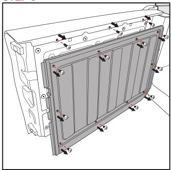
• Remove the 10 screws from the liner panel on the wider half of the tailgate as shown with appropriate tool. Then remove the 3 inner screws that are along the top of the of tailgate.
