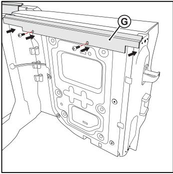
• Screw on tailgate rail G using the 2 factory screws again, along the top of tailgate.
