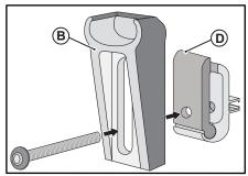
• Attach the Clamp to the Patented Adjustable Bar Bracket as shown.
