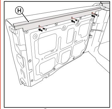
Screw on tailgate rail using the 3 factory screws again, along the top of the tailgate.
