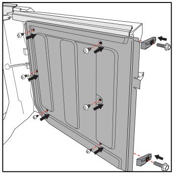
• Screw on the liner panel with the 6 factory screws again. Then screw back the 2 bump stops again as shown.
