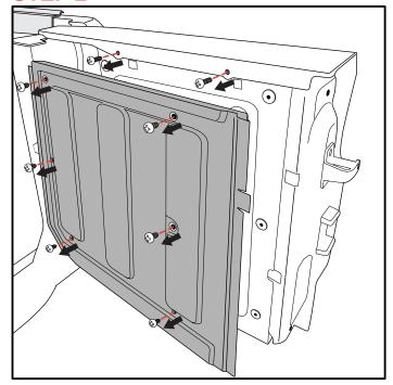
Remove the 6 screws from the liner panel as shown with appropriate tool. Then remove the 2 inner screws that are along the top of the of tailgate.
