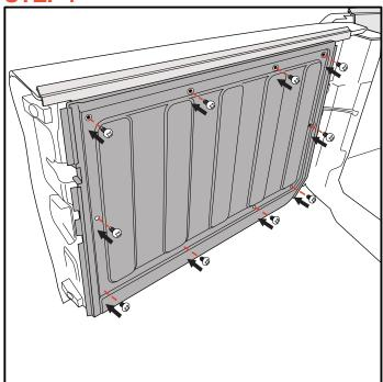
• Screw on the liner panel with the 10 factory screws again.
