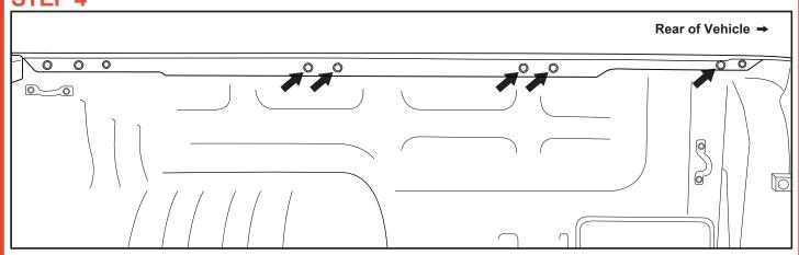
• Remove the 5 screws as shown from both inner sides on the tub, using appropriate tool.
