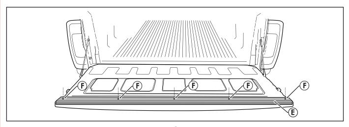
• Remove the red tape from back of the Tailgate Rail E. Then stick the Tailgate Rail centrally onto the tailgate. Drill with a 4mm drill bit through the 5 holes and then rivet F the Tailgate Rail to the tailgate.
