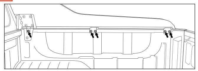
• Remove the five factory screws pointed above with T45 torx bit.
