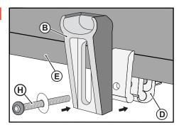
• Slide and attach the Patented Adjustable Bar Bracket (B) to aluminium on the Rails (E) as shown using M8 Bolt with washer (H) and Side Clamps (D).
