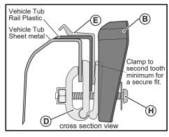
• Engage the Adjustable Bar Bracket (B) to Front Side Rails (E) as shown in order on the left. Repeat for opposite side.
