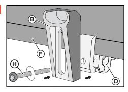
• Slide and attach the Patented Adjustable Bar Bracket (B) to aluminium on the Side Rail (F) as shown using M8 Bolt with washer (H) and Side Clamps (D).
