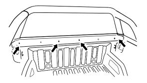
Note: There a 6 holes in the front of the vehicle's tub. Only 4 of these holes are used.
