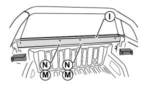
• Insert the M8 screws (M) and M8 washer (N) to hold the front rail in place.
