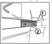
Remove Bolts **2** & **1** to loosen and remove the sport bar bracket before attaching Front Rail.
