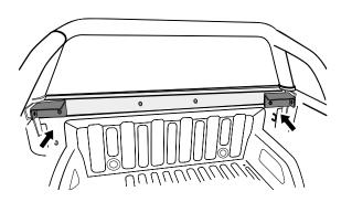
• Prior to installing the outer-most M8 screws (M), re-install the sport bar bracket (1) infront of the front rail (1).
