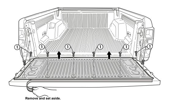
• Remove the inspection panel by unscrewing any remaining screws 2.
