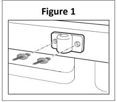
(c) Fit the Support Bars according to Section 3 of this Instruction.
