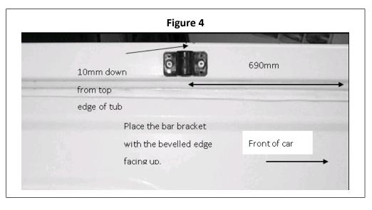
(c) Repeat for other side of tub. Use instruction over page to fit tonneau support bar.
