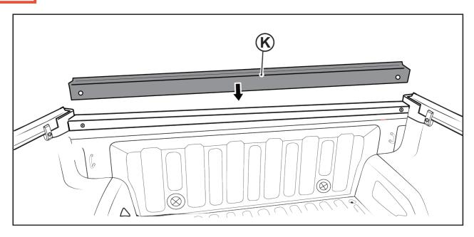
• Place the front aluminium rail onto the front rail of the vehicle's tub and ensure the 2 bolt holes line up with the holes in the aluminium
