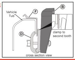
• Engage the now assembled Bar Bracket & Clamp to the Side Rails as shown in the next steps.
