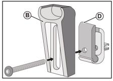
• Attach the Clamp ① to the Patented Adjustable Bar Bracket ⑥ as shown.
