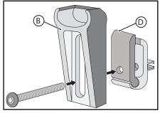
• Attach the Clamp D to the Patented Adjustable Bar Bracket B as shown.
