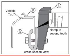
• Engage the now assembled Bar Bracket & Clamp to the Side Rails as shown in the next steps.
