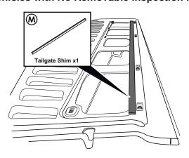
• If there is no inspection panel on the vehicle, peel the backing off the adhesive tape, attached to Tailgate Shim (M). Then position directly below the cage nuts - ensuring distance between the two is no greater than 1mm.
