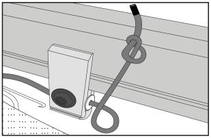
• Rethread the washer and tie the end of the rope in a knot.
