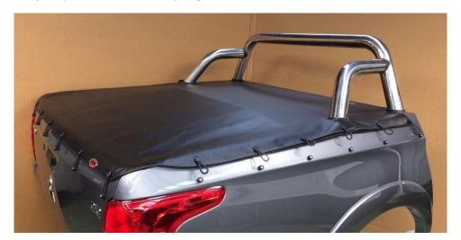
**14.** To Fit Anti-Abrasive Discs: Firstly clean the area behind each bunji head with a clean rag and methylated sprits. Then attach the anti-abrasive discs centrally behind each bunji head.
