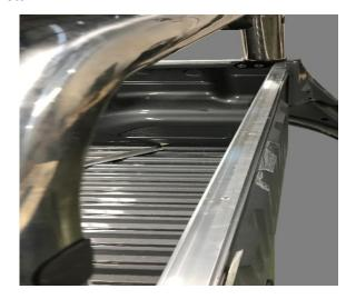
**3.** Sit and centralize the 20 x 20mm angle on top of the 50 x 25mm angle. The 20mm face will face forwards towards the cab. Drill 5 evenly spaced holes through the smaller angle, into the larger one already fitted. The first hole needs to be 30mm from each end.
