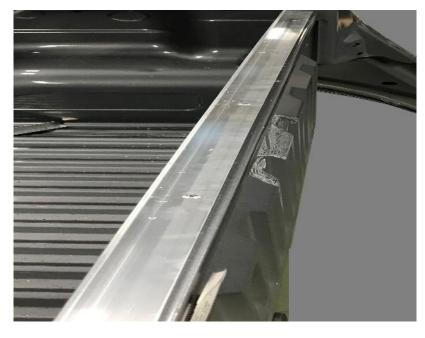
**3.** Sit and centralize the 20 x 20mm angle on top of the 50 x 25mm angle. Drill 5 evenly spaced holes through the smaller angle, into the larger one already fitted. The first hole needs to be 30mm from each end.
