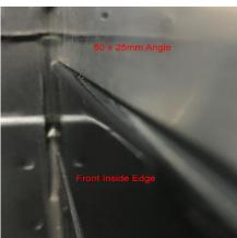
2. Drill 5 evenly spaced holes through the 25mm section of the angle and into the top edge of the tub. The first hole from each end will be about 50mm from the end of the angle. Pop rivet into place with 5 x long rivets.
