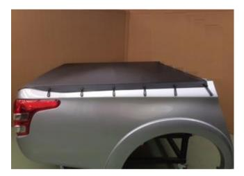
**15.** To Fit Anti-Abrasive Discs: Firstly clean the area behind each bunji head with a clean rag and methylated sprits. Then attach the anti-abrasive discs centrally behind each bunji head.
