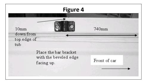
**Step 3. Fit The Buttons To Vehicle**
