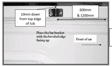
**Figure 2**: Placement of bar bracket
