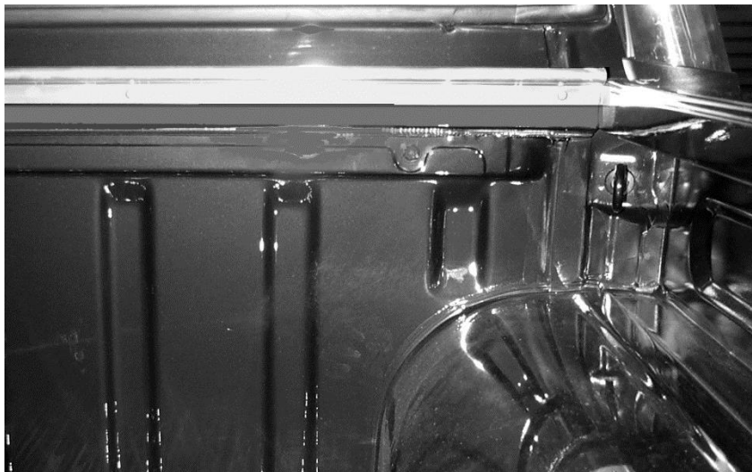
Figure 1: Placement of aluminium rope track. Ensure channel is above the tub's top edge.
