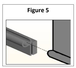
(e) To fit the rope buttons to the sides:
