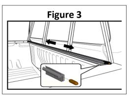
(f) Rivet the aluminium rope track into position.
