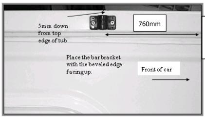
Figure 2: Placement of bar bracket
